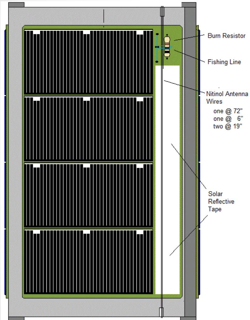
on command to deploy the antennas which are stowed for launch, the burn resistor heats, melting the nylon fishing line holding the wire antennas
